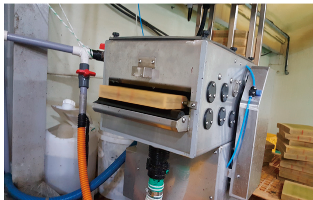
Fig. 2. Washer for sponge in dried-laver Pyropia sp. processing.
