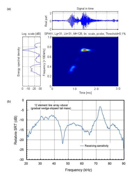
Fig. 5. Time-frequency representation of received chirp pulse signal (a) and relative receiving sensitivity (SRT) (b) for the linear array acoustic transducer without a series matching inductor  $L_s$  (Fig. 2).
