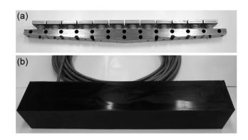
Fig. 1. Photographs of a linear array acoustic transducer with a gradual wedge-shaped tail mass after (b) and before polyurethane molding (a).
