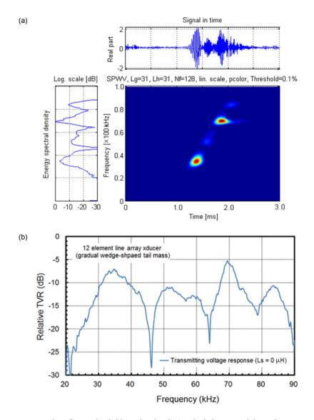
Fig. 4. Time-frequency representation of transmitted chirp pulse signal (a) and relative transmitting voltage response (TVR) (b) for the linear array acoustic transducer without a series matching inductor  $L_s$  (Fig. 2).
