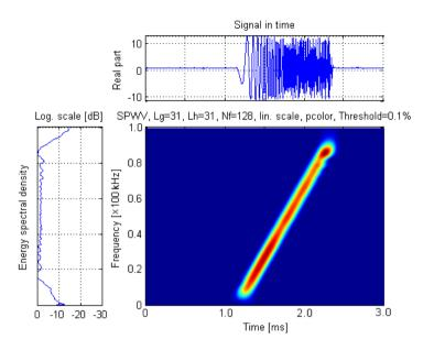
Fig. 3. Time-frequency response characteristic of chirp pulse signal at the electrical terminal of a linear array acoustic transducer (Fig. 1).
