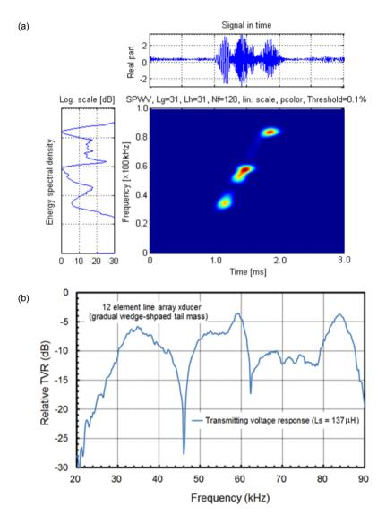
Fig. 9. Time-frequency representation of transmitted chirp pulse signal (a) and relative transmitting voltage response (TVR) (b) for the linear array acoustic transducer with a 137  $\mu$ H series matching inductor (Fig. 2).
