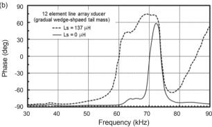
Fig. 8. Comparison of the input electrical impedance patterns without (solid line) and with a 137  $\mu$ H series matching inductor (dot line).
