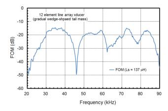
Fig. 10. Compensated FOM (figure of merit) performance curve for the linear array acoustic transducer with a 137  $\mu$ H series matching inductor (Fig. 2).
