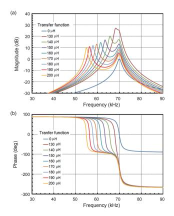
Fig. 7. Comparison of the calculated transfer functions of the compensated and non-compensated linear array acoustic transducers for tuning conductance  $L_s$ = 0-200  $\mu H$ .
