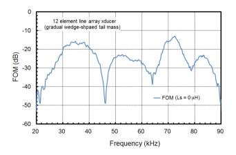
Fig. 6. FOM (figure of merit) performance curve for the linear array acoustic transducer without a series matching inductor  $L_s$  (Fig. 2).
