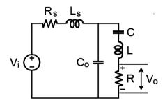
Fig. 2. Compensated electrical equivalent circuit of a linear array acoustic transducer (Fig. 1) with a series matching inductor.  $V_i$ , input voltage;  $V_o$ , output voltage;  $R_s$ , driving impedance;  $L_s$ , matching inductance;  $C_o$ , clamped capacitance; C, capacitance;  $C_s$ , inductance;  $C_s$ , resister.
